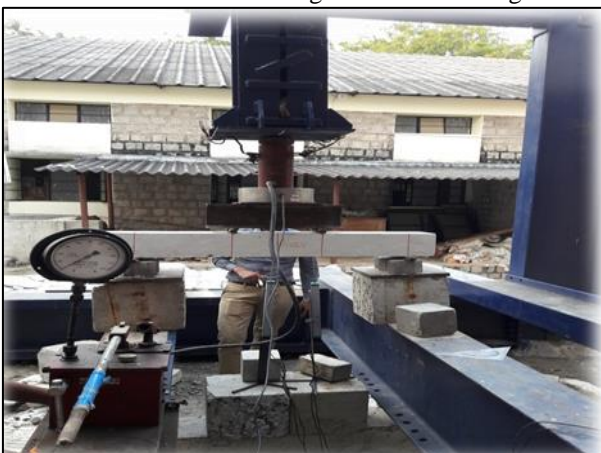
Fig. 1: Set up of a GPC beam under two-point
