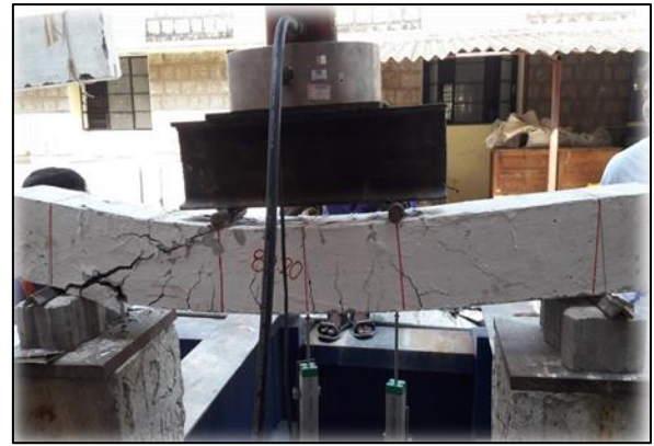
Fig 2: Flexural failure of a beam under two-point loading
