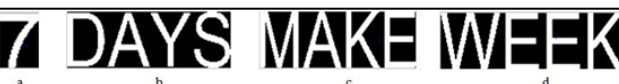
Fig. 3.8: Word Segmentation of second line of English Text (a) First Word (b) Second Word (c) Third Word (d) Fourth Word
