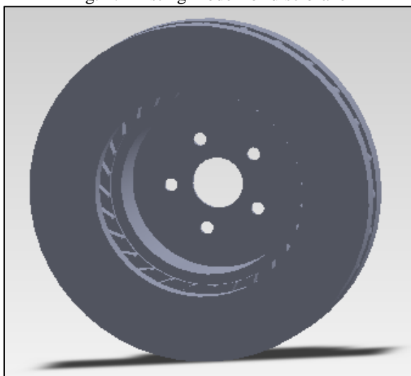
Fig. 2: Modified Model of disc brake
