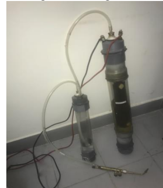
Fig.10: Actual setup of efficient welding torch by hydrogen fuel cell
