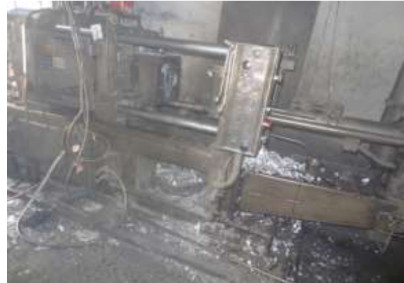
Fig. 7: 120-Tone Cold chamber die casting machine
