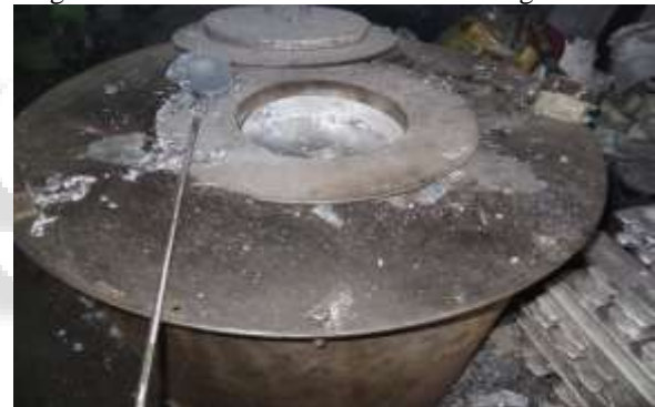
Fig. 8: Aluminium melting furnace
