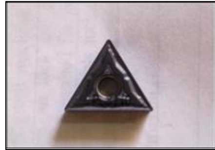
Fig. 3: PVD coated carbide insert
