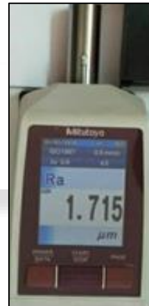
Fig. 4: Surface roughness tester showing Ra Value
