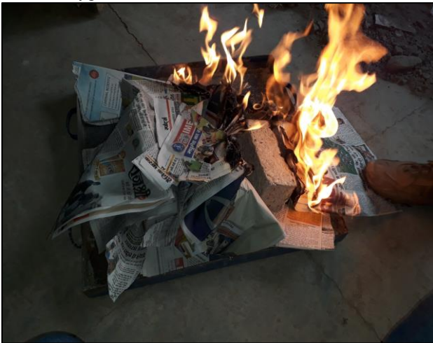
Fig. 4.4: Brick after burning for five minutes
