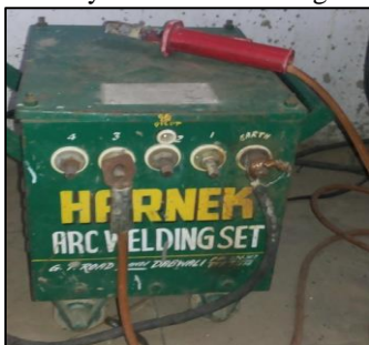
Fig. 1: Manual metal arc welding machine
