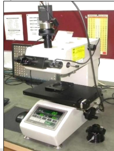
Fig. 8: Vickers hardness testing machine
