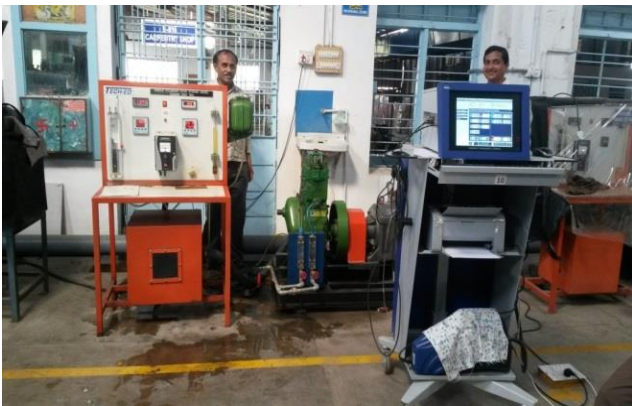
Fig. 3: Diesel Engine Test Rig with AVL DiTEST (Exhaust gas analyzer)
