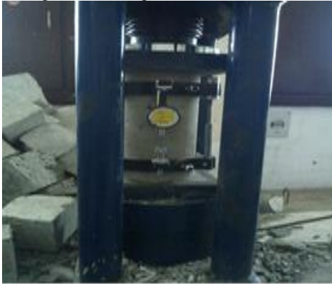
Fig. 6: Testing of cylinders for modulus of elasticity
