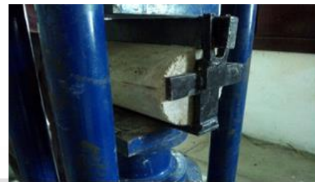
Fig. 4: Split tensile strength test
