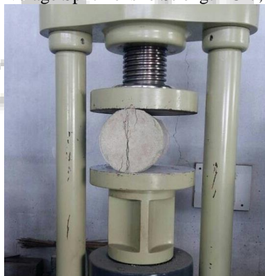
Fig. 7: Failure Pattern of Cylinder
