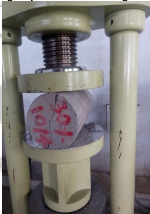
Fig. 6: Failure Pattern of Cylinder
