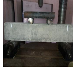
Fig. 8: Failure Pattern of prism
