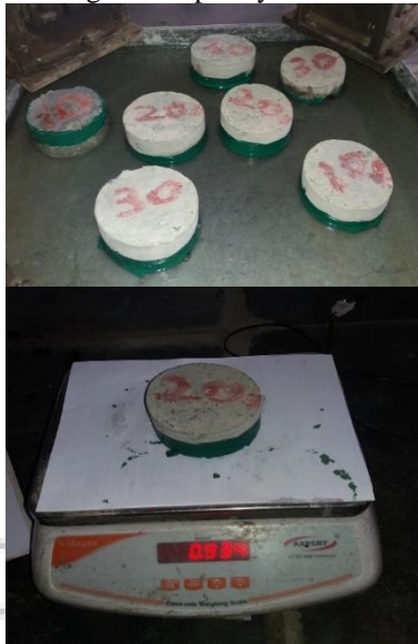
Fig. 10: Test Setup For Sorptivity
