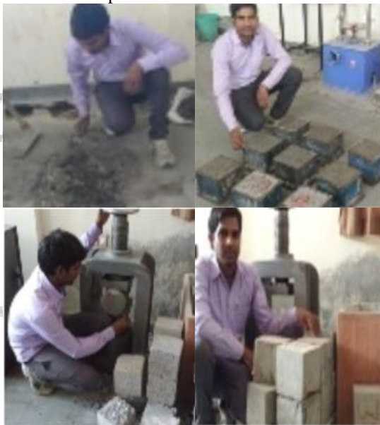
Fig. 2: Mixing of concrete and concrete cubes
