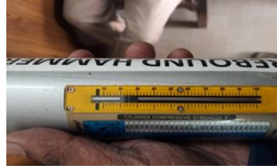
Fig. 3(a): Reading (2)of rebound hammer
