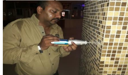
Fig. 4: Field test with rebound hammer
