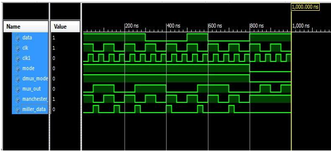
Fig. 6: Simulation result for proposed a) Manchester and b) Miller encoder.
