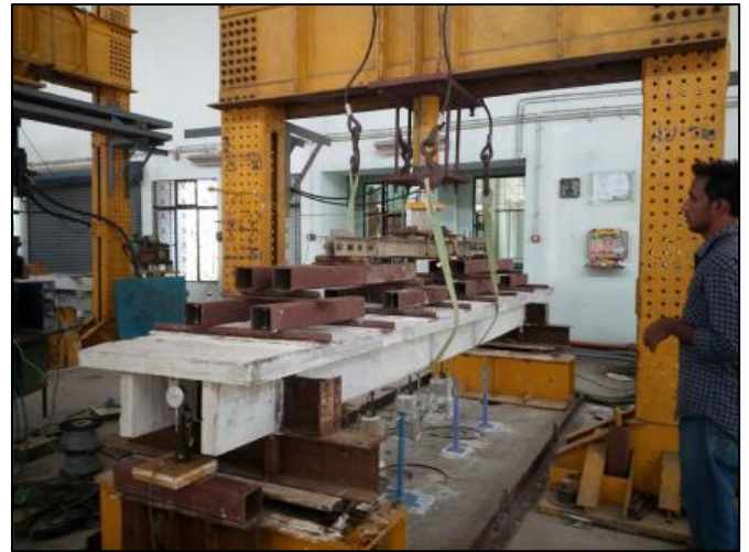
Fig. 7.b: Testing of precast ferrocement roofing
