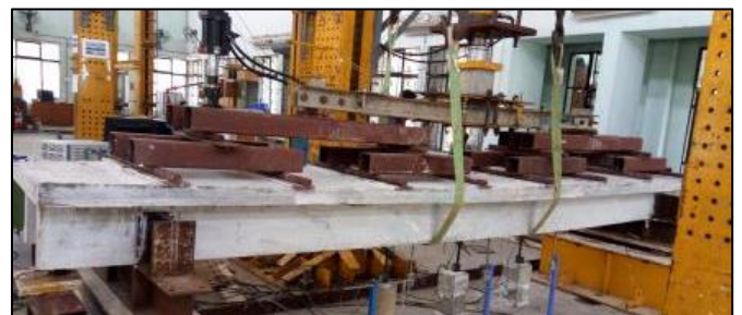
Fig. 9: Failed specimen, after ultimate loading
