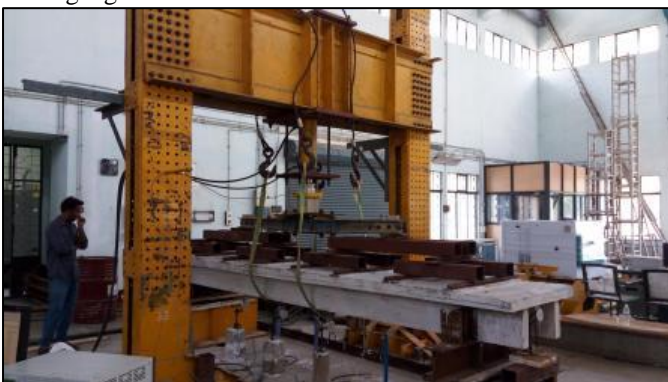
Fig. 7.a: Testing of precast ferrocement roofing
