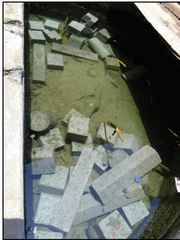
Fig. 4: Curing of Cubes, Prisms, and Cylinders
