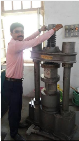
Fig. 5: Testing of Concrete Cube Samples
