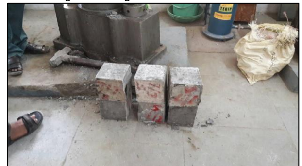
Fig. 3: Demoulded Concrete Cube Samples
