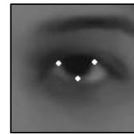
Fig. 9: Corner points after applying Harris Corner Detector
