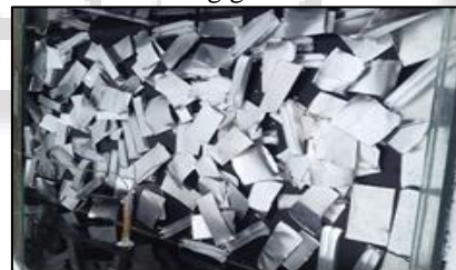
Fig. 5: width wise double slope modified solar still material using aluminum
