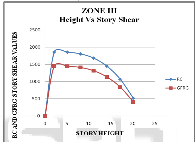
Fig. 35: A Graph with Story Height Vs Story Shear of RC and GFRG buildings for a load combination of 1.5(DL+EQ-X) for ZONE III.
