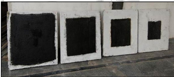
Fig. 5: Prepared specimen with increasing bond area by 25, 50, 75 and 100% the slab area.
