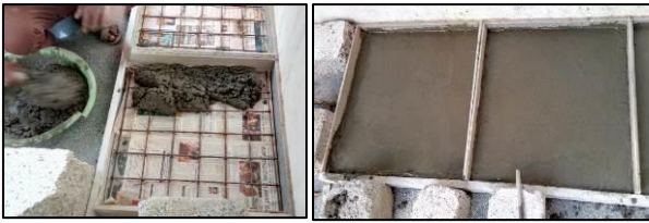
Fig. 2: Casting (a) and finished surface(b).
