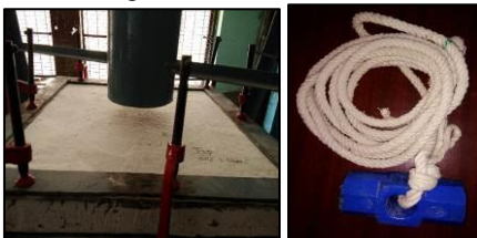
Fig 6: Testing specimen with c-clamps (a) and hammer of 10 pounds connected with rope (b).
