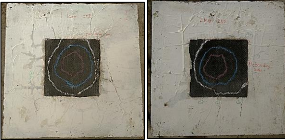
Fig. 9: Failure of 25% wrap one and two layer bottom view.
