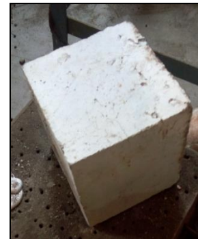
Fig. 2: White patches on sample after heating
