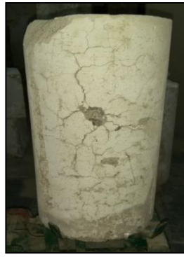
Fig. 4: Cracks on sample after heating
