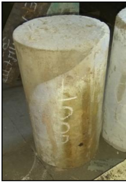
Fig. 3: Yellow patches on sample after heating.
