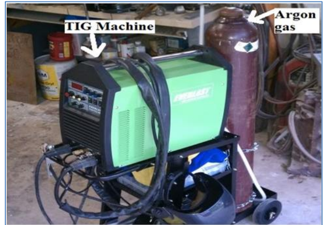
Fig. 4.1: TIG Welding Setup— Ever last TIG 250 AC/DC TIG Welding System.
