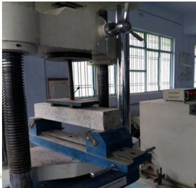
Fig. 3: Beam on Universal Testing Machine
