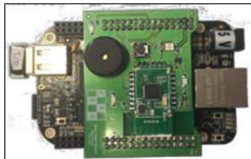
Fig. 3: Gateway: shield placement on the BeagleBone Black.
