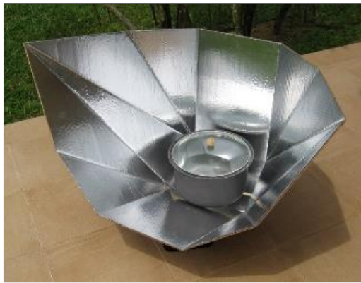
Fig. 2: Panel Solar Cooker.
