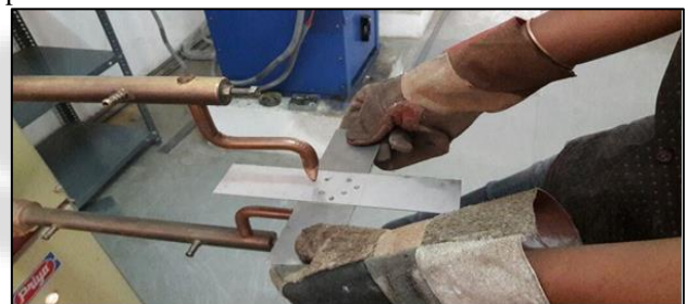
Fig. 4.4: Spot welding of cross joint of sheets
