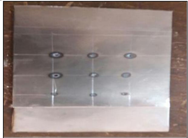
Fig. 4.3: Spot welding of lap joint of sheets
