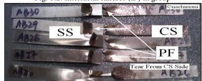
Fig 1.3 Tear from one side (PF) failures in group
