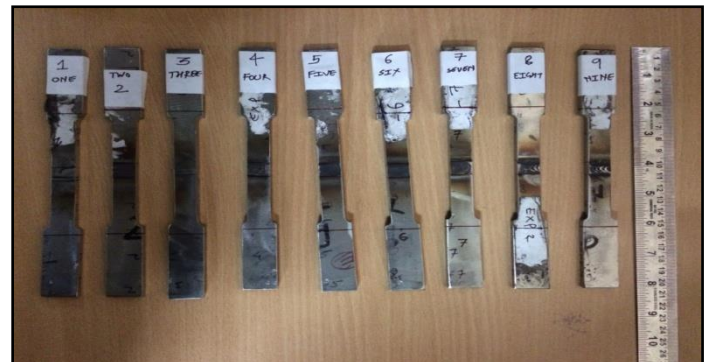
Fig. 7: Machined Sample used for Tensile test
