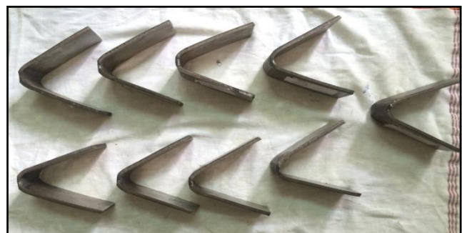
Fig. 12: Samples After Bending Test
