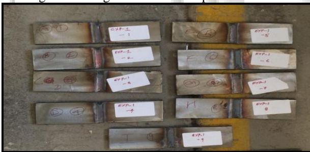
Fig. 3: Welded Samples of Stainless Steel
