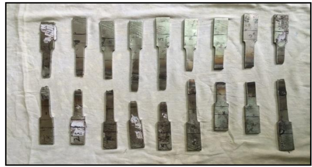
Fig. 10: Weld Samples after Tensile Test
