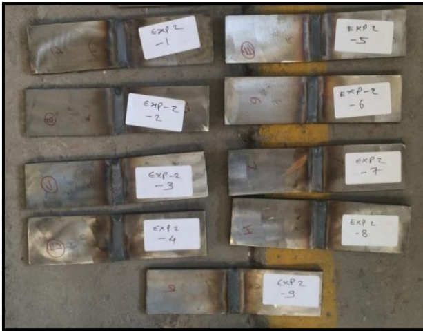
Fig. 8: Samples Prepared for Bending Test
