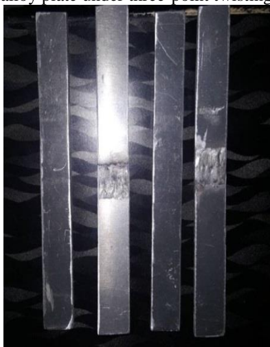
Fig. 1: The specimen for testing welded and unwelded
