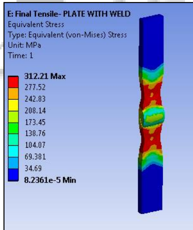
Fig. 23: Tensile test with weld simulation result
