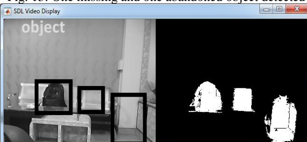
Fig. 14: One unattended and two missing objects detected
