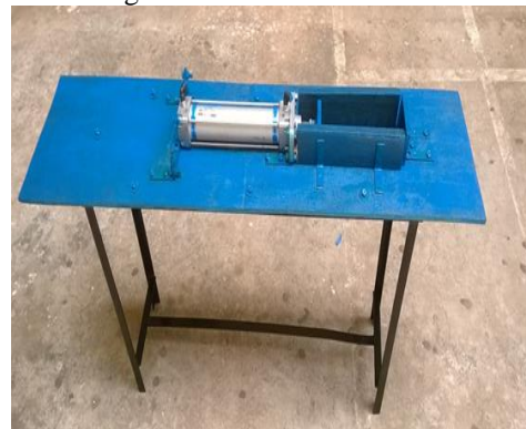
Fig. 10: Working of Pneumatic Can Crusher
