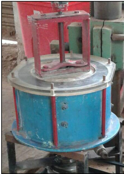
Fig. 2: Experimental setup of pot tester
