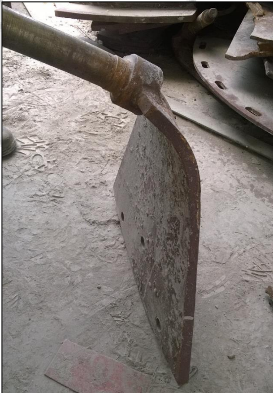
Fig. 3: Deformed blade after working
