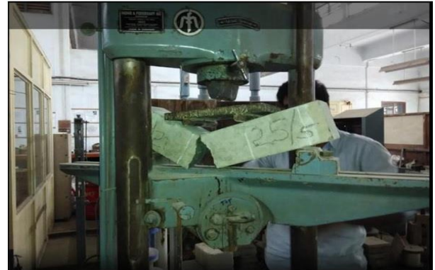
Fig. 12: Testing of prisms in Universal testing machine
