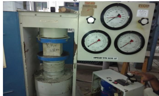
Fig. 6: Testing of cubes in Compression testing machine
