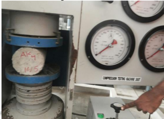
Fig. 9: Testing of cylinders in Compressive testing machine
