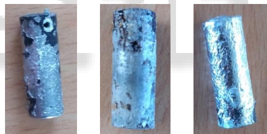
At 550°C 10min 500°C 5min 450°C, 1min Fig. 6: Samples annealed at different temp. And time
