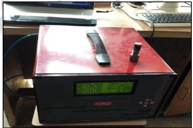
Fig. 3: Exhaust gas analyzer
