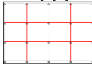
Fig. 3: Plan showing highlighted partition walls
