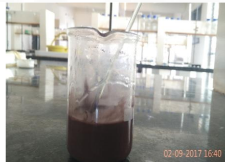
Fig. 4: 0.1% of Copper added to 99.9% of Epoxy resin
