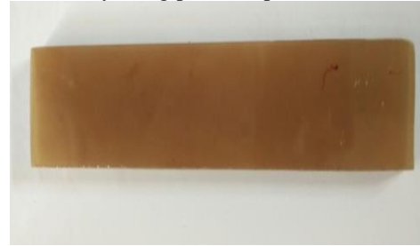
Fig. 8: Rectangular specimen for bending moment
