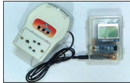
Fig. 6: Energy meter which displays the power consumed by a device
