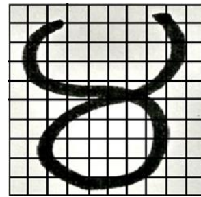
Fig. 5: Character image is divided into 10x10 zones for computing the directional features.
