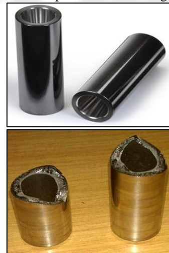
Fig. 2: Photograph of a New Piston pin and damaged piston pin
