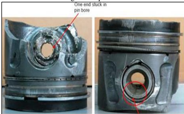
Fig. 4: Pin shear and broken piece
