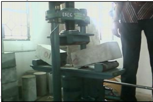
Fig. 9: Failure of Beam
