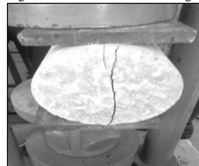
Fig. 7: Failure of Cylinder
