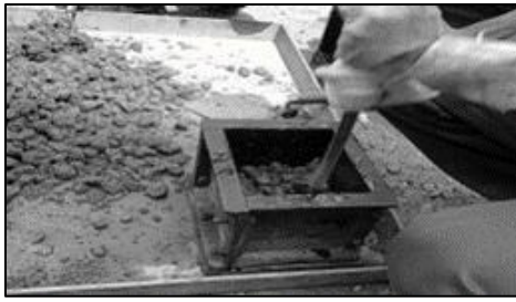
Fig. 2: Casting of Concrete Cube
