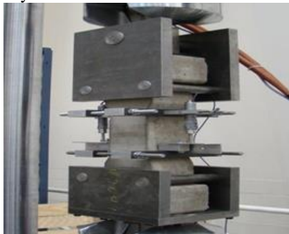
Fig. 1b: Geometry and Dimensions of the Direct Tensile Specimen Used at UT-Arlington [Chao et al, 2011]
