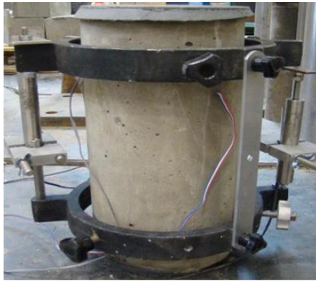
Fig.1c: show Test setup for obtain Compressive Stress-strain relation
