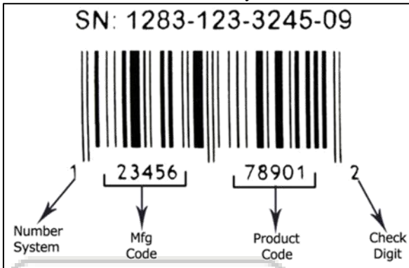
Fig. 4: Structure of barcode
