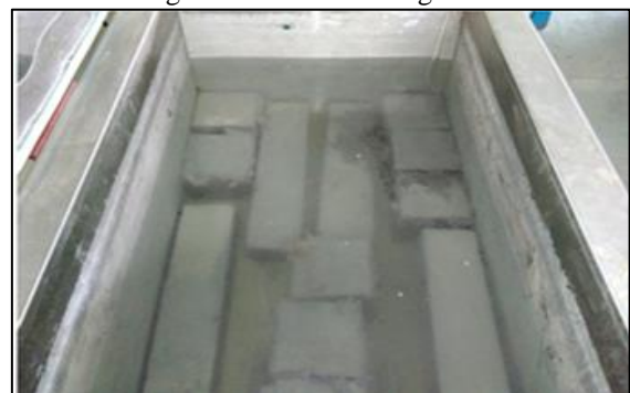
Fig. b: Beam Sample Curing
