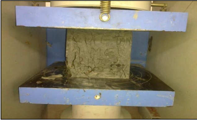
Fig. 1: Compressive strength test
