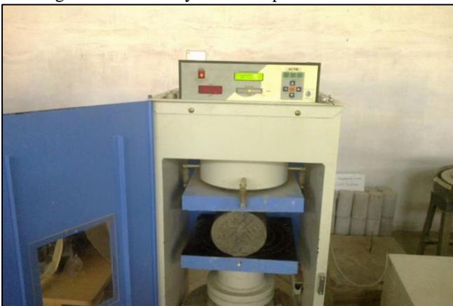
Fig. 2: Split tensile strength test
