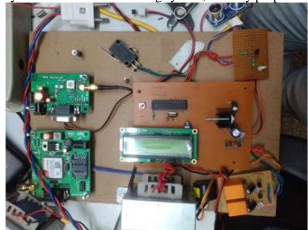
Fig. 4: circuit of vehicle monitoring system
