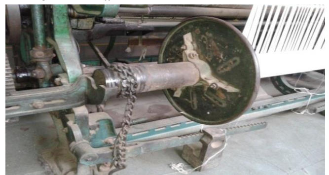
Fig. 3 Conventional Negative Let-Off Motion
