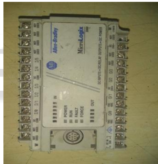
Fig. 1: PLC Micro logix1100 ( 4 I/P and 4 O/P)
