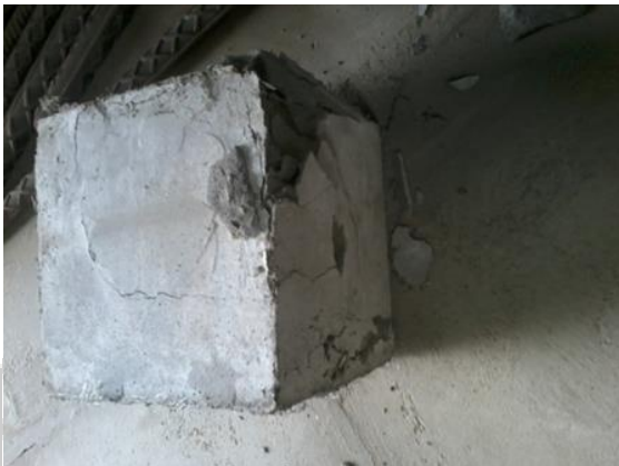
Fig. 2: failure load cube
